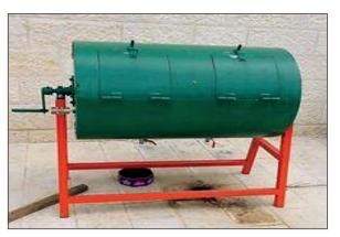
Figure 1. The used rotary drum compost (reactor)
